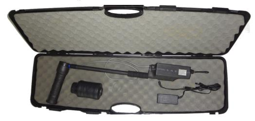
The Bandit is a non-intrusive pig signaler which uses either permanent magnets or active transmitters mounted onto the pig to detect passage from 0.022 to 45.73 mph (0.01m/s to 20 m/s). With thousands of systems have used around the world over the past 15 years, the pig signaler has developed a strong reputation in the industry for its reliability and durability in even the harshest environments.
